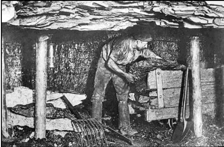
A miner filling a typical Wooden Tram, Tub (local name) or Jottie at the coal face. Note the safety lamp hanging on the roof support, which would have only provided very poor lighting.
